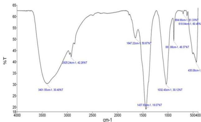
Fig. 3: FT-IR analysis of biosynthesized ZnO NPs
