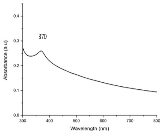
Fig. 1: UV–VIS spectrum of biosynthesized ZnO NPs
