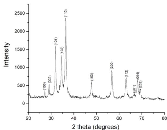
Fig. 2: XRD spectra of biosynthesized ZnO NPs
