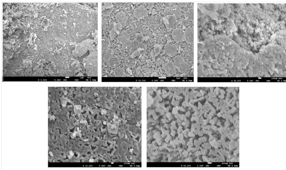
**Fig. 4:** SEM images of biosynthesized ZnO NPs using corn silk
